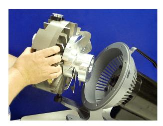
4. Remove pump module from the frame.
