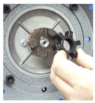
4. Insert spider in motor coupling.
